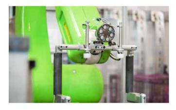
in the market. There are several components that weigh more than seven or ten kilograms, "laboratory robots" could not compete. The FANUC robot, which is based on the M-20*i*A series, has a reasonable reach of 1.813 mm regarding industrial applications.
